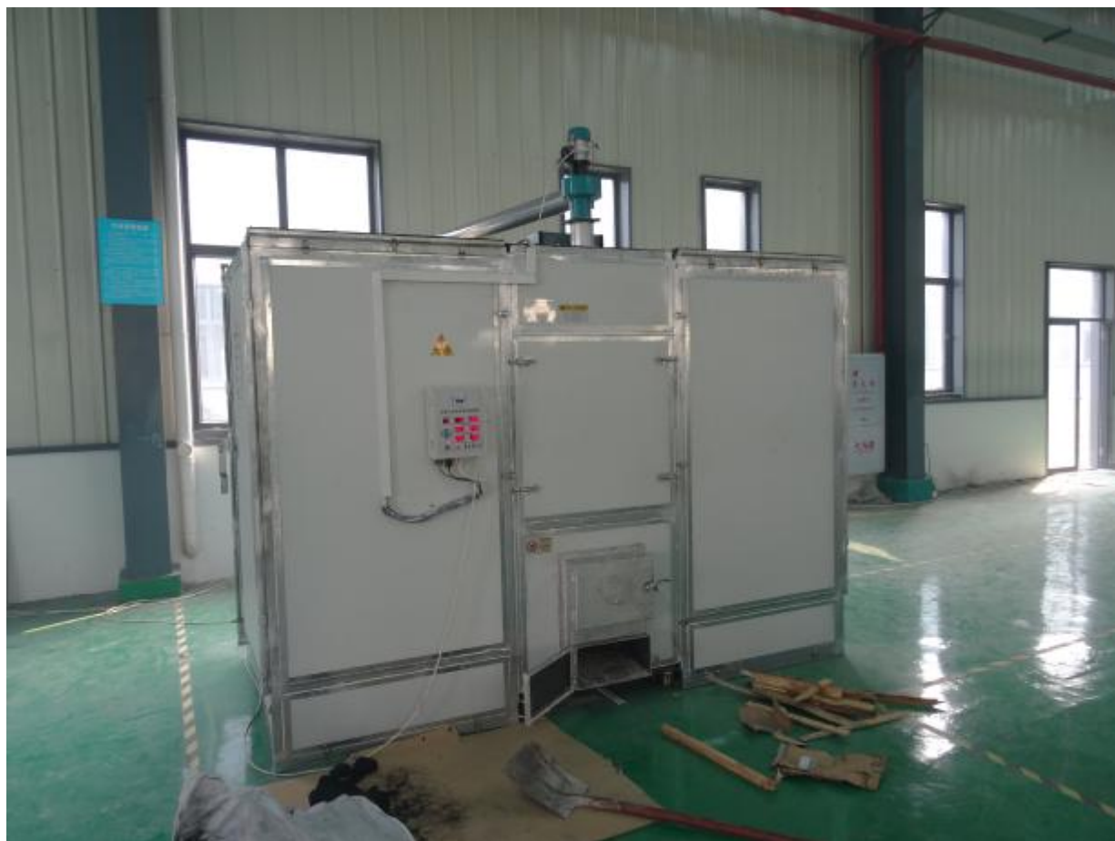
5HGS-6.2-RL 型果蔬烘干机样机图片
